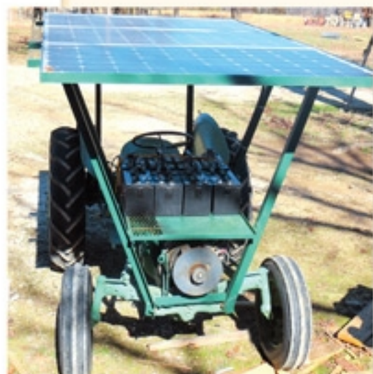
An Arkansas couple retrofitted this 1950 Ford tractor with solar panels and eight batteries.
